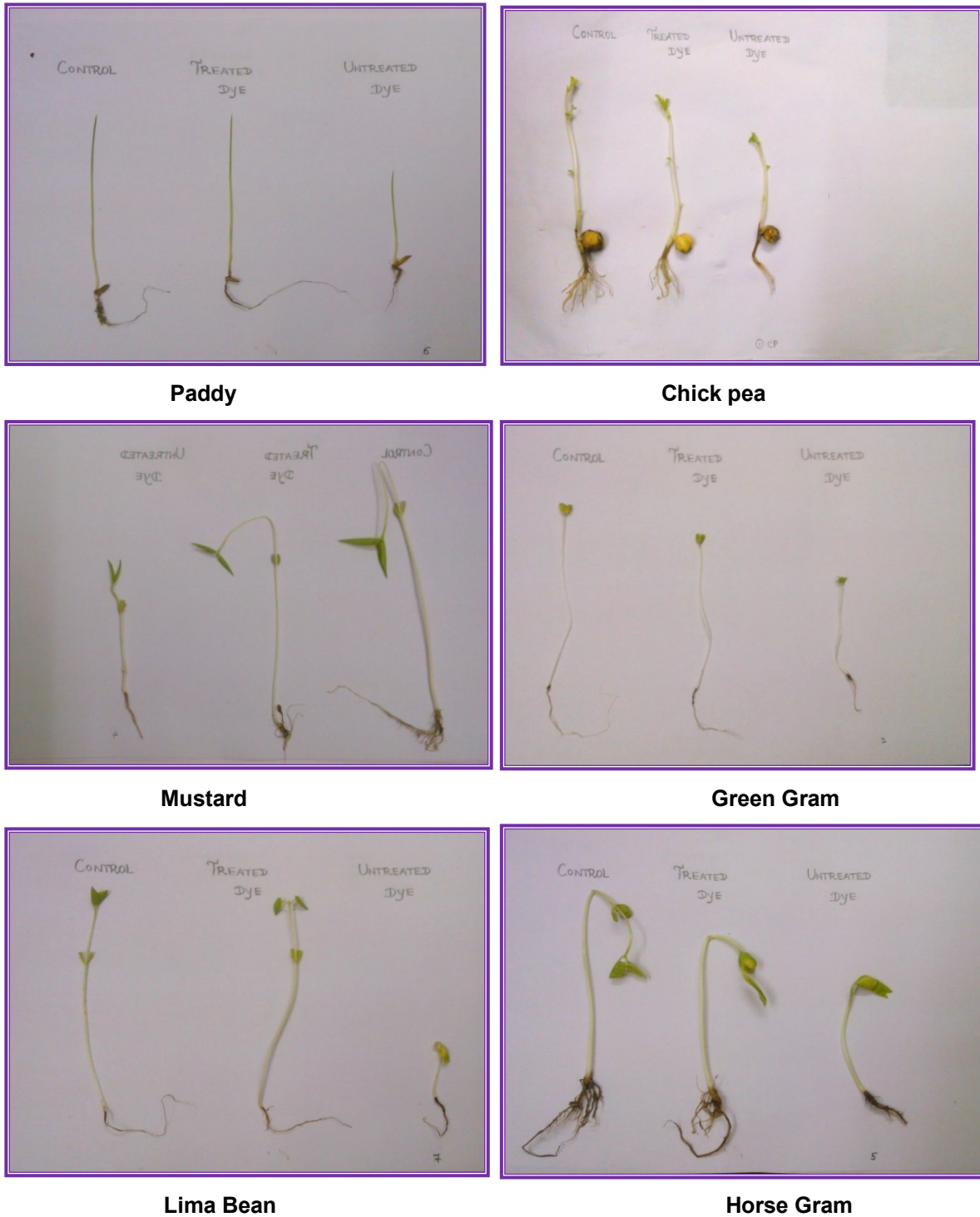
Figure 12: Phytotoxicity analysis of control, untreated and treated effluent sample
