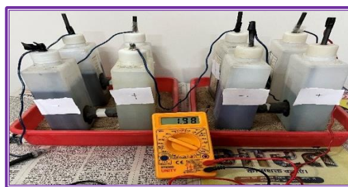
Figure 1A: Schematic Diagram of Series Connection Figure 1B: MFC setup of Series Connection
