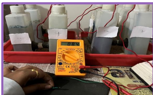
Figure 4A: Electricity Generation by Multiple Chamber Connected in Hybrid Connection
