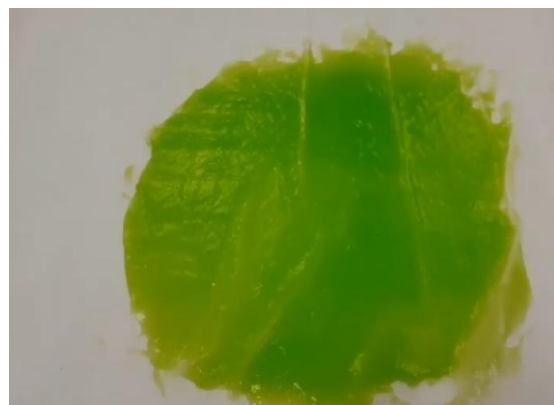
Fig 1: Spread bioplastic sheet on bake paper
