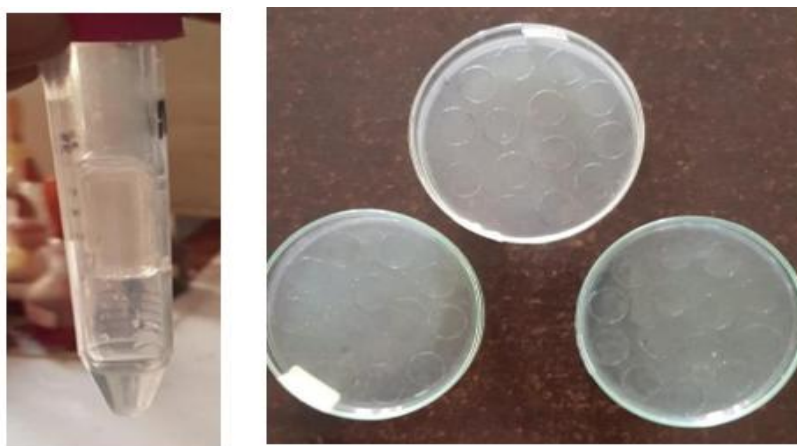
Figure 1: Ultrafiltration tube where nanoparticles were filtered from medium (left), Petridish containing ocusert formulation embedded with drug loaded nanoparticles (right).
